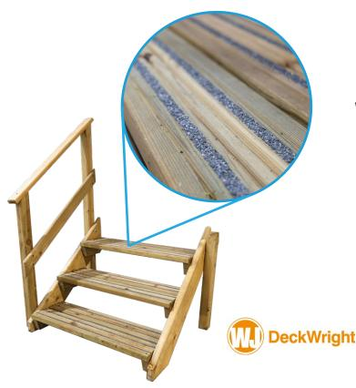
Each of the grooved boards consist of two anti-slip strips enhancing user safety. To be classed as 'non-slip decking' the PTV (Pendulum Test Value) minimum requirements are 35.
